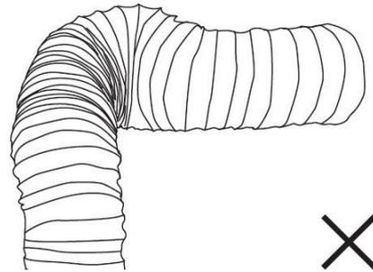
For internal motor units ,please install Semi rigid ducting with the least amount of bends possible, maximum length of Semi rigid ducting should be no longer than 5 meters.
